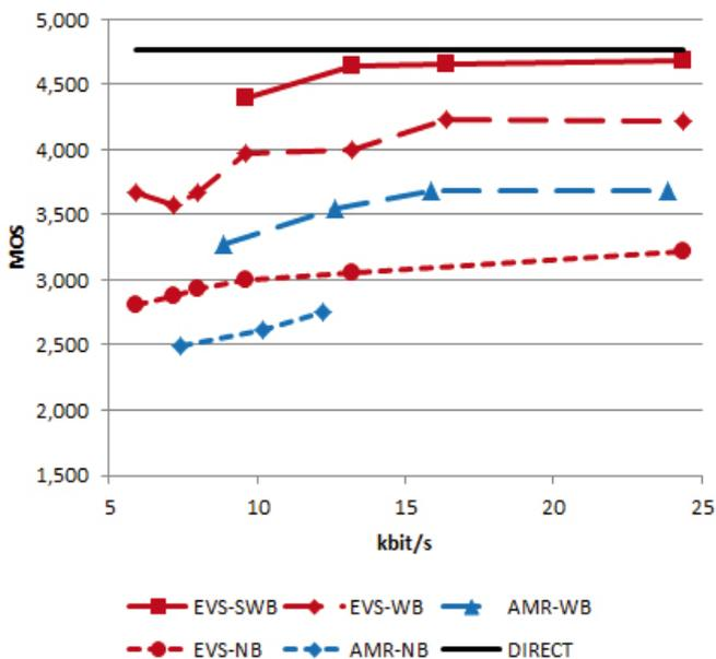
Figure 3: 3GPP EVS characterization test results for multi-bandwidth clean speech
